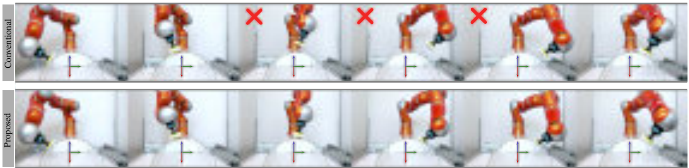
Fig. 6. Experiment #3a: Fast surface polishing scenario is illustrated by controlling the contact on curved surface. The motion sequence for the conventional method (top row) and the proposed approach (bottom row) are shown. The contact is lost during high-velocity phases (marked with red \times ) due to velocity-dependent dynamical coupling effects within the conventional approach; see the video attachment.
