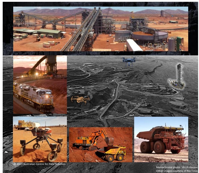
Fig. 1. Scope of mining automation encompasses mine, rail and port operations. Robotic platforms and data analytics are being used increasingly in high-tech open-pit mines [4]. Examples include autonomous drills, haul trucks, shovels, conveyors, drones, trains and ships.
