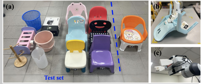
Fig. 4. Experiment Details. (a) Robot Experiment Data. The right chair is used for parameter tuning. The rest 12 objects are previously unseen and are used for testing our method. (b) A test chair with handles attached under the seat. (c) The end effector is mounted with two RGB-D cameras for scanning and tracking respectively.
