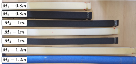
Fig. 5: Foam bars with different lengths and materials that have been used in the real experiments.
