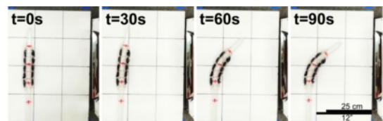
Fig. 11. The robot can steer towards the heat source within 90 s.
