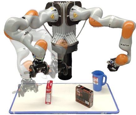
Fig. 1: A 7-degree-of-freedom manipulator carrying a weight in a cluttered environment with uncertain tracking control.
