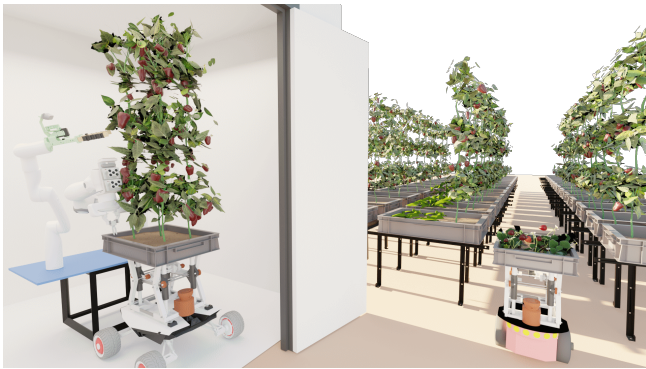
Fig. 2: Modified Pioneer 3DX and omnidirectional Agilex Scout robots with a lift mechanism. Robots navigate between the growing pods to transport plants to the manipulator workstation. The raised growing pods simplify navigation within a known and static environment. Treating plants on a remote location enables tight packing of the growing pods.
