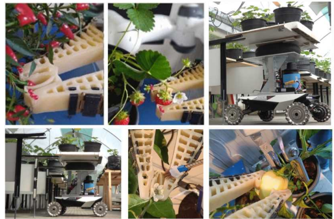
Fig. 11: Showing the dual arm manipulation system picking various fruit, pollinating flowers, and pruning the plant. We are showcasing the results of our first experiment, growing 60 sweet peppers, 60 hot peppers and 40 strawberries, demonstrating the feasibility of the proposed system.
