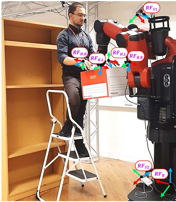
Fig. 4. Experimental setup for naturalistic object handover of the big-sized box bimanual handover from robot-to-human while the human is standing on the ladder, annotated with the defined coordinate systems.
