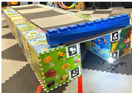
Fig. 16. The straight tunnel with a squared cross-sectional shape of 0.6 m edge length for flight tests.
