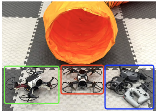
Fig. 15. The autonomous tunnel flight system (red frame), the tunnel flight system in [6] (green frame), and the commercial DJI Avata FPV system for manual flights (blue frame).
