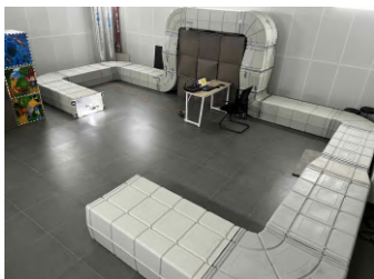
(f) Rigid vent pipe with various cross-section sizes and sharp turns.
