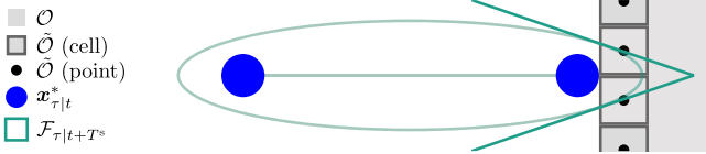
Fig. 5. Visualization of a scenario in which the robot would crash into the obstacle if the constraints are not tightened. The obstacle is inflated, here represented by \mathcal{O} , with corresponding occupied grid cells \tilde{\mathcal{O}} and the point representation of \tilde{\mathcal{O}} in the code. While the ellipsoid does not intersect the grid points, it overlaps with the obstacle region, i.e., \mathcal{F} \cap \mathcal{O} \neq \emptyset .
