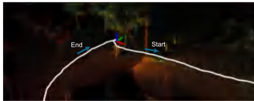
Fig. 5. For loop -sequences, the start pose and the end pose are the same.
