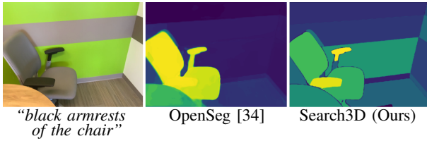
Fig. 3: Pixel-level features. OpenSeg [34], used in OpenScene, has a limited understanding of finer-grained object parts in the scene. We propose to obtain pixel-aligned features by combining Semantic-SAM segments [47] and SigLIP [32], enabling fine-grained localization of concepts such as object parts and materials. Bright yellow means higher similarity to the text query.
