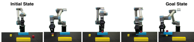
Fig. 5. Given an initial environment configuration in the first column, our model can generate an action sequence reaching the goal state.
