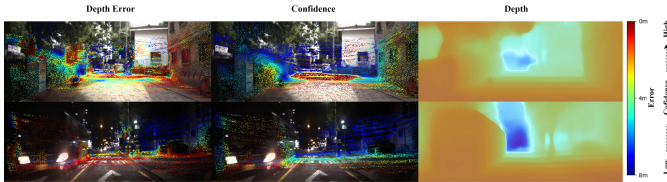
Fig. 4: Predicted confidence and depth error on MS 2 dataset [9]. Left to right: depth error overlaid on the image, confidence overlaid on the image, and predicted RGB depth.
