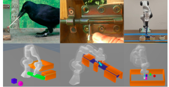
Fig. 1: (Top) Examples of tool manipulation in nature: a crow using a tool to obtain food [5] and manipulating a sliding bolt latch, alongside a Franka Panda robot performing an analogous obstacle removal task. (Bottom) Complex manipulation scenarios solved by our proposed approach: tool-assisted object retrieval through pushing and picking, latch mechanism manipulation, and tool-based obstacle removal.
