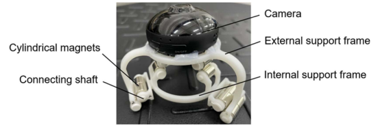
Fig. 5. Overview of tip mount design.
