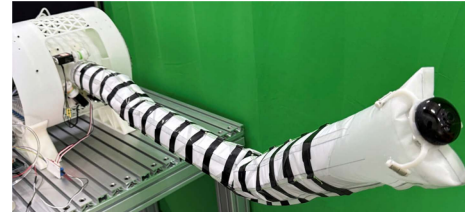
Fig. 1. Snapshots of MLSGR demonstrating its ability to counteract its own weight while carrying a tip-mounted sensing device in various postures.
