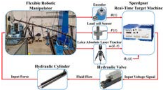
Fig. 6. Experimental Platform of the Flexible Manipulator.
