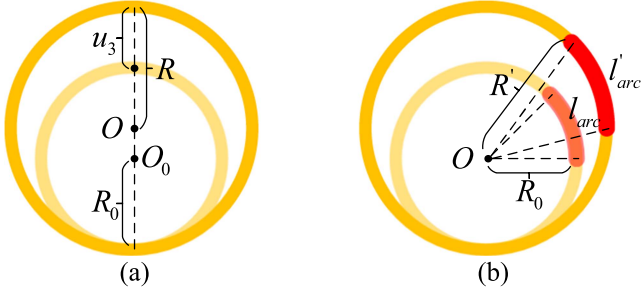
Fig. 7. Schematic diagram of the relationship between radial displacement u_3 and circumferential strain \varepsilon_2 .
