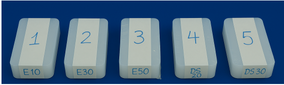
Fig. 2. Soft material samples composed of gel or silicone, numbered from 1 to 5 in increasing stiffness. E: Ecoflex™ 00-10, 00-30, 00-50; DS: Dragon Skin™ A-20, A-30. This figure has been edited for clarity.
