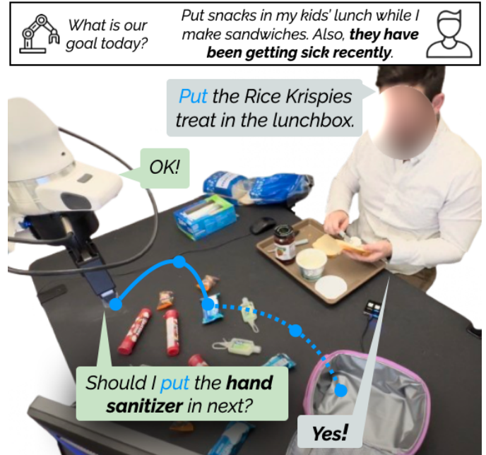
Fig. 1. We present ProVox (“Proactive Voice”), a framework for personalization and proactive planning in the context of situated human-robot collaborations. In the first phase of a collaboration [Top], a human communicates their goals and distinct preferences, enabling the robot to personalize . Throughout the rest of the collaboration [Bottom], the robot continues to incorporate and anticipate their partner’s intent to proactively suggest helpful actions (e.g. “Should I put the hand sanitizer in next?”) ahead of explicit instruction, reducing the user’s mental load while they assemble the sandwich.
