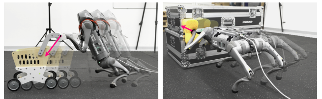
Fig. 5: Snapshots of two whole-body loco-manipulation tasks, where the desired EE force are overlaid as pink arrows. Upper: pushing a shopping cart while walking in bipedal mode; bottom: holding a sponge while walking in quadrupedal mode.
