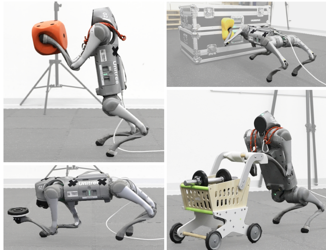
Fig. 1: Various whole-body loco-manipulation tasks enabled by RAMBO on Unittree Go2 [25] in both quadrupedal and bipedal modes.
