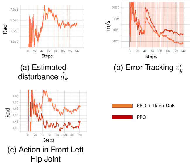
Fig. 7. Lateral force test on the robot body at steps 4k and 8k, and its effects on the front left hip joint action and body velocity error.
