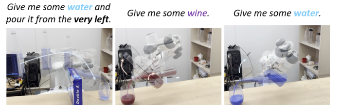
Fig. 9. Pouring motions performed by a 7-DoF Franka Panda robot, where inverse kinematics (IK) are solved to obtain joint trajectories from the generated SE(3) pouring trajectories.
