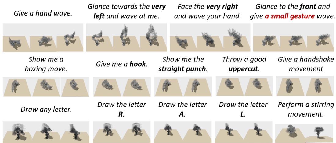
Fig. 12. Correct 7-DoF robot arm motions generated by MMFP from text inputs. Diverse motions are produced from less specific commands (e.g., “Give a hand wave”, “Show me a boxing move”, “Draw any letter”), while more detailed texts yield accurate, specified motions. MMFP effectively captures complex task-motion dependencies, even in multi-task scenarios. Example videos: Waving, Boxing and Handshake, and Drawing and Stirring.
