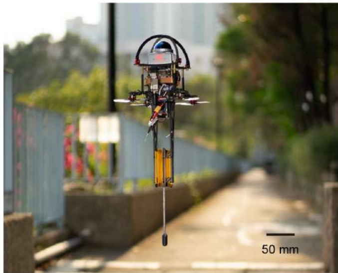
Fig. 1. A 220 g thrust-based hopping robot constructed from a quadcopter (160 g) and a passive leg (60 g) demonstrating an ability to carry a 730 g LiDAR payload for mapping applications. Despite a thrust limit of only 440 g, the hopper is able to carry as much as 2 kg.
