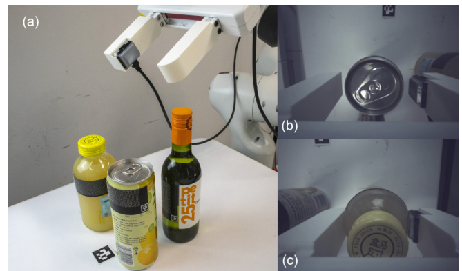
Fig. 13: Manipulation with limited vision information. (a) The robot is tasked with aligning the direction of labels on all the bottles. (b)(c) The robot efficiently adjusts the orientation of the bottles by rotating its wrist joint, even if the labels on the bottle are not visible from current perspective. The grasping pose is estimated through a simple combination of TacTape and diameter measurement.
