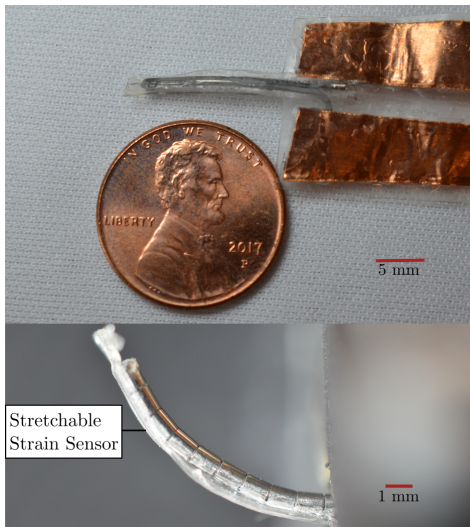
Fig. 5. (Top): ELMNT® stretchable strain sensors installed onto a notched tube wrist [30]. The sensing area measures 17 mm in length and 0.6 mm in width, with a trace width of 0.3 mm.
