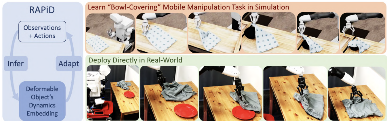
Fig. 1: RAPiD: Rapid Adaptation of Particle Dynamics (Left) is a method for learning to perform real-world deformable object mobile manipulation tasks by inferring and adapting to the unknown dynamics of deformable objects in real-time. Top Right: In simulation, RAPiD first learns a visuomotor policy to achieve a deformable object mobile manipulation task, such as bowl-covering, by inferring the deformable object’s dynamics from the robot’s visual observations and actions. Bottom Right: RAPiD then deploys the learned visuomotor policy directly to the real world to achieve the deformable object mobile manipulation task, under unseen object dynamics, instances, categories, and lighting conditions , using only onboard sensor signals.
