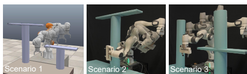
Fig. 15. Universality of URPlanner across different manipulators and environments. Scenario 1: training a KUKA robot. Scenario 2: training a Franka robot in a simple environment. Scenario 3: training a Franka robot in a complex environment.
