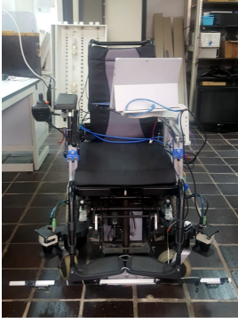
Fig. 2: Intelligent wheelchair with the set of sensors used in the localization module.
