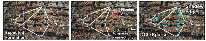
Fig. 1: Illustration of the proposed multi-robot cooperative localization in a large-scale deployment scenario. Here, the links shown in “White” are the edges of the sparsely-connected sensing and/or communication graph, in the Ground Truth frame. The second figure depicts the estimates, where the line in “Red” represents ‘flipping’ of estimates due to the sparse graph setting. We add new ‘shadow edges’ (depicted in “Blue”) from inferred information to recover the relative locations (right figure).
