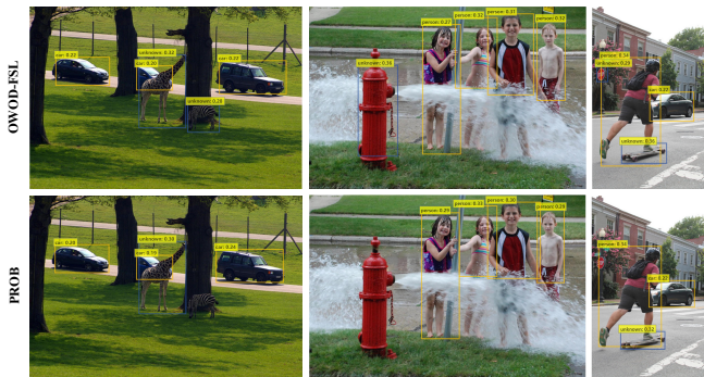
Fig. 3. Unknown detection comparison: OWOD-FSL (top) vs PROB (bottom). Yellow/blue boxes mark known/unknown objects. OWOD-FSL detects more unknowns (zebras, hydrants, stop signs) with higher confidence (e.g., skateboards), proving better open-world robustness.
