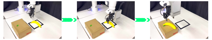
(a) Picking and placing an unseen banana with Franka + Robotiq 2F-85 gripper \mathbb{G}_5 (Base manipulator + New task requirements).
