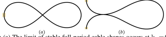
Fig. 5: (a) The limit of stable full-period cable shapes occurs at k_c = 0.908 , which forms a figure eight. (b) The limit of non self-intersecting cable shapes occurs at k_{max} = 0.855 , at which the full-period elastica just touches itself.
