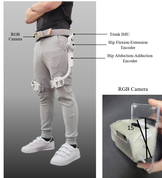
Fig. 1. Lower-limb wearable hip complex assist robot MoonWalk.Omni with integrated RGB camera for visual perception
