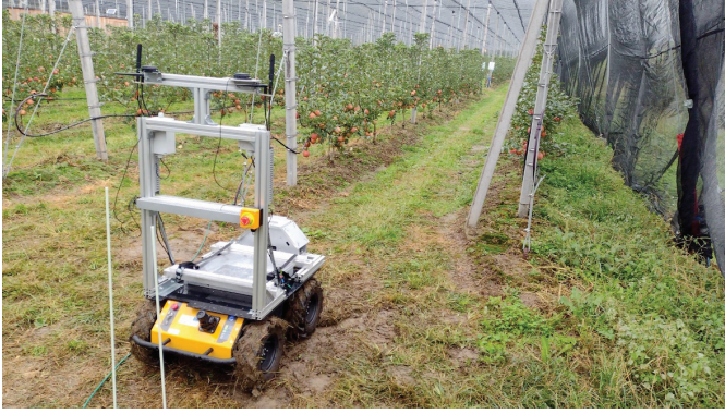
Fig. 1. The experimental area, consisting of an apple orchard with 2.7 m wide and 25 m long rows. The robot has been tested under various weather and terrain conditions, such as dry sunny days and tall grass, as well as muddy terrain conditions in rainy and cloudy weather (as shown in picture).
