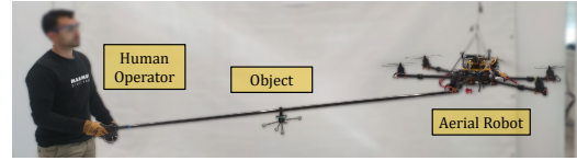
Fig. 1. Collaborative transportation task of an object between a human operator and an aerial robot.
