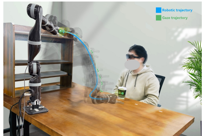
Fig. 1. Experimental setup of the proposed gaze-based teleoperation approach. This approach utilizes gaze data to guide the freeform movement of the robotic manipulator. A Gaussian Mixture Regression (GMR) model is employed to infer the operator's intended robotic movement and mitigate motion fluctuations caused by involuntary eye movements.
