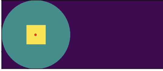
Fig. 4. A visualization of the primary sensor slewing capability. The satellite is traveling towards the right edge of the figure, which indicates the extent of onboard lookahead sensor data. The primary sensor is pointed at nadir, which is indicated by the red dot. The yellow area shows the reachable set of observation targets that the primary sensor can be slewed to within one cycle (4 seconds) of slewing time. The turquoise blue area shows the entire primary sensor range, which is determined by the primary sensor's 15^\circ maximum off-nadir angle. The purple area represents observation targets that have been sensed by the lookahead sensor but could not be reached during this cycle regardless of the initial position of the primary sensor.
