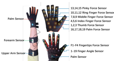
Fig. 2. Data glove with angle sensors and force sensors.
