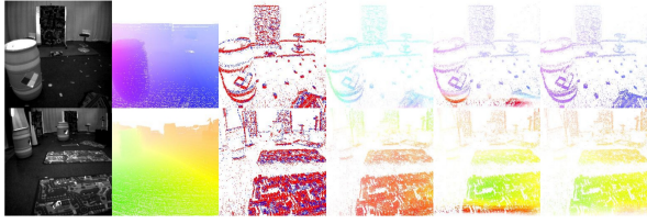
Fig. 6. Qualitative visualization of flow estimation on the indoor_flying sequence. From left to right: reference frame, ground truth, stacked events, EVFlow [18], BFlow [12], and Ours. For better visualization, all estimated flow maps are masked to show only regions where events are triggered.
