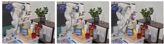
Fig. 13: Whole-body collision avoidance with GeoPF. (a) Planner with no avoidance, naturally leading to multiple collisions, (b) End-effector-only avoidance fails to avoid elbow collisions. (c) GeoPF's whole-body geometric-aware collision avoidance successfully modulates arm and end-effector trajectories to safely avoid all obstacles.
