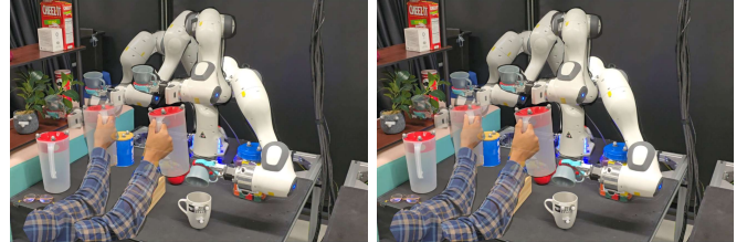
Fig. 1: Reactive robot behaviour in unstructured, cluttered, dynamic environments. The robot transfers and pours the tea from the shelf to the cup (left), then returns the set while reacting to a human dynamically moving objects (right)—requiring accurate geometric representations for real-time motion adaptation.
