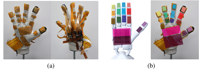
Fig. 6: (a): Tactile sensor layout on the Shadow Hand: palm side (left, sensor-covered) and dorsal side (right, no sensors). (b): Regions for tactile readings mapping. Same-color blocks mark corresponding regions.
