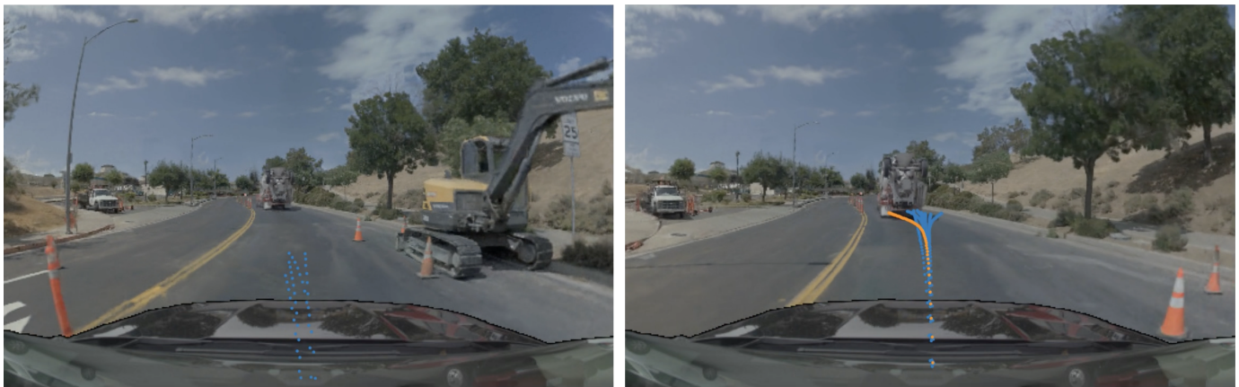
Fig. 9. In a challenging closed-loop simulation of a construction scene, the baseline DINOv2-based model (left) stops in the middle of the road and does not start driving again, whereas our triplane-based model (right) has no difficulty nudging around the parked excavator and driving behind the cement mixer. On the front camera views are the predicted ego-vehicle trajectories (selected driving trajectory in orange, with the other 5 predicted trajectories in blue).
