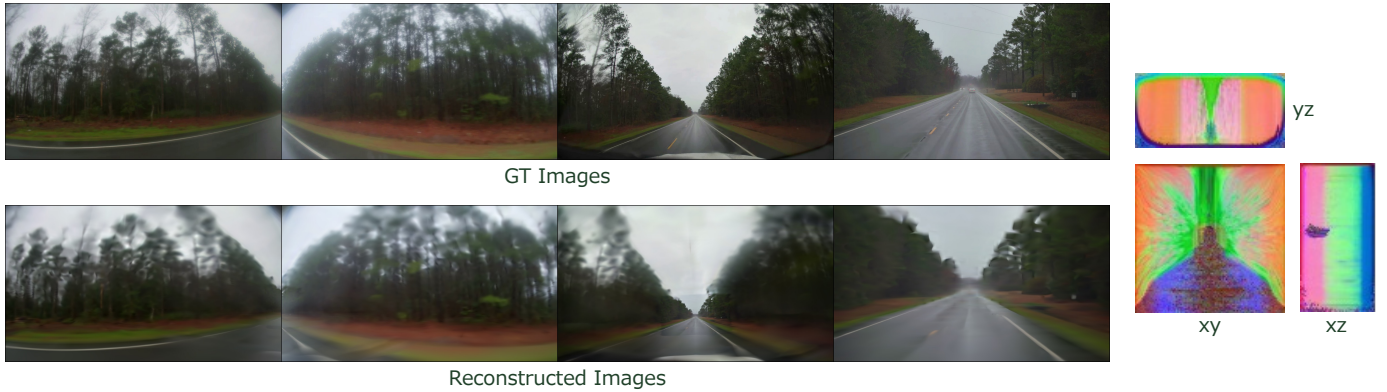
Fig. 7. Triplanes can faithfully represent higher resolution data without requiring any changes to triplane sizes. Since these cameras are all front-facing, the rear half of the xy and xz planes are unused.
