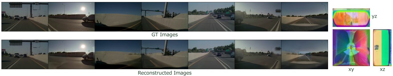
Fig. 4. Triplanes can accurately represent environments observed by outward-facing cameras ( top ), producing accurate reconstructions ( bottom ) and semantically-meaningful features after only being trained with self-supervised pixel reconstruction losses ( right , a PCA visualization of triplane features).
