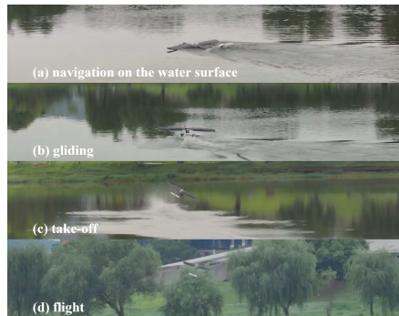
Fig. 10. Transition from water to air.
