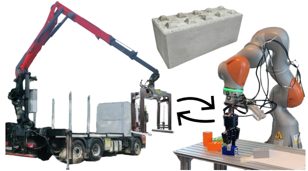
Fig. 1: Motivation: articulated boom crane with concrete block (left) and developed laboratory-scale setup (right) as a testbed for autonomous assembly.
