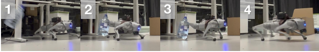
Fig. 5: Balancing under external disturbance . The robot is subjected to a lateral push at the trunk and subsequently recovers from the perturbed posture, reestablishing balance.
