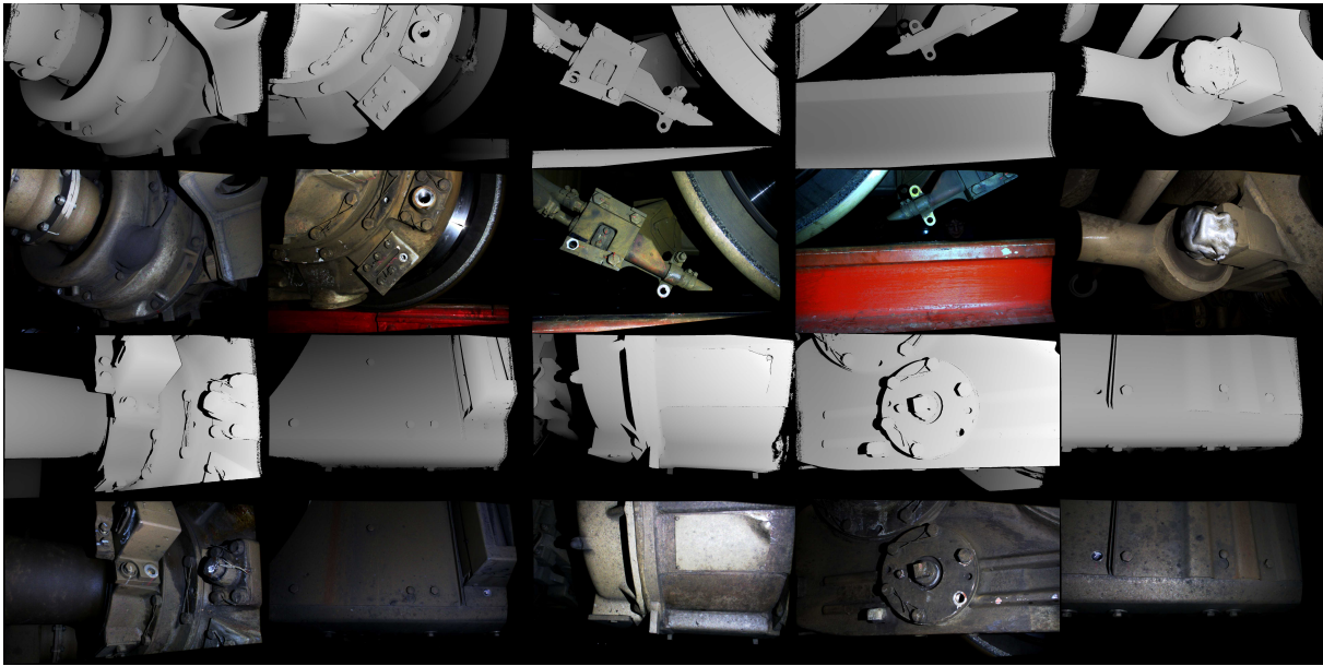
Fig. 2. A display of the dataset captured by the robot. The 1st and 3rd rows are depth maps, and the 2nd and 4th rows are the corresponding RGB images
