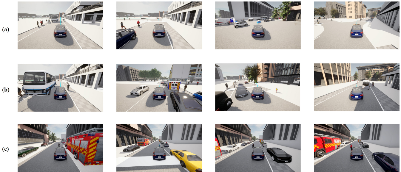
Fig. 5: Qualitative examples of the proposed proactive trajectory planning framework: (a) Normal driving scenario, (b) Scenario with surrounding participants, (c) Ghost-probe scenario, the red bounding boxes indicate the potential ghost-probe zones.
