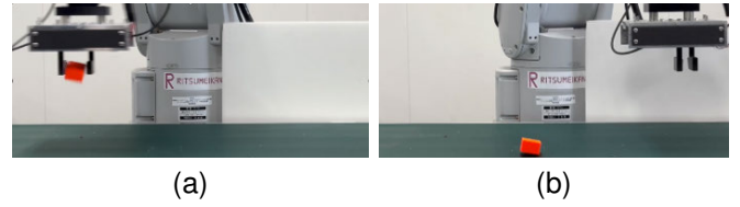
Fig. 11. Experimental snapshots for the scenario without stiffness anisotropy but under the high translation acceleration of a_{a,m} = 5.2148 \text{ m/s}^2 : (a) gripper began translating the object, and (b) object was dropped.
