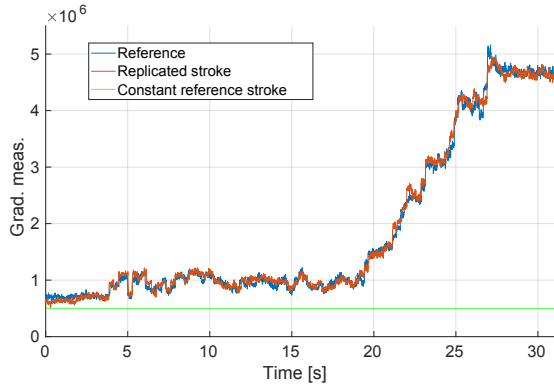
Fig. 6. Demonstrated scraper bending angle reference for a simple linear stroke along with the executed values recorded during the stroke replication with the proposed robotic system. For comparison, the same stroke is also executed with the constant reference value of 5e^5 (see also Fig. 5).
